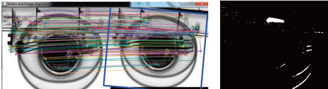
Figure 6: Automatic detection of an irregularity by comparison with reference image: registration process and indication on a difference image
