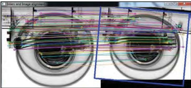
Fig. 8. RANSAC filtering and transform computation.
