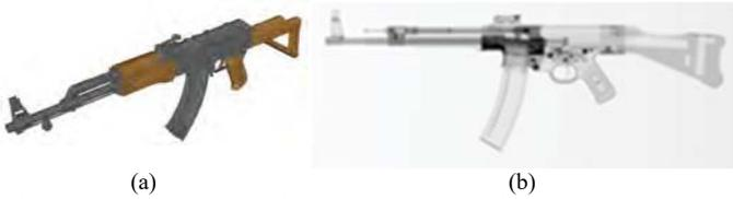
Fig. 4. 3D CAD model (a) and the simulated 2D X-ray projection (b).
