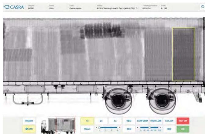
Fig. 14. The *Customs Simulator* is a computer-based training and testing tool that is capable of simulating ATR functions.
